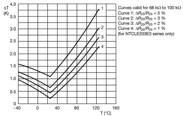
TEMPERATURE DEVIATION AS A FUNCTION OF THE AMBIENT TEMPERATURE
